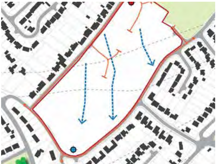
SuDS Constraints and Opportunities Diagram ● High point ➡ Direction of flows ● Low Point - - - - - Existing combined sewer
