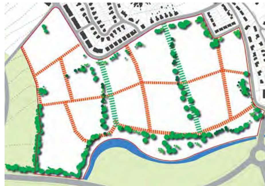
Street structuring for gravity surface drainage
